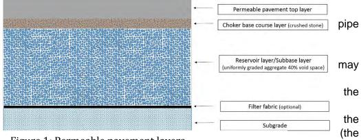
Figure 1: Permeable pavement layers
